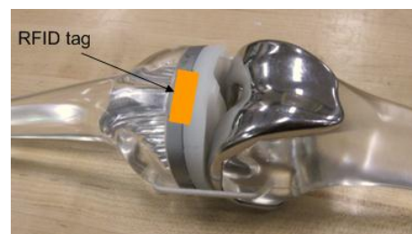
Fig. 1. RFID tag on an orthopedic implant.
