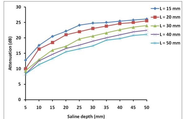
Fig. 4. Signal attenuation without metal sheet using 10 mm interior electrodes with different distances between electrode center (L).
