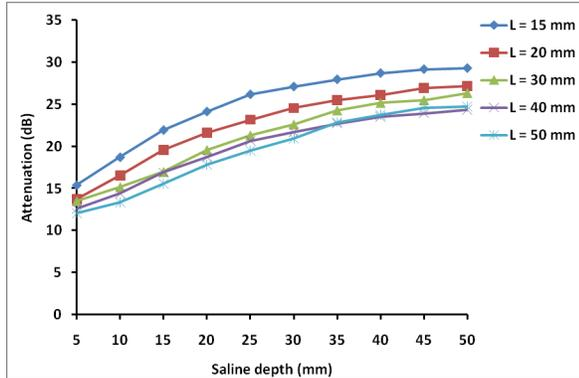
Fig. 6. Signal attenuation with metal sheet using 10 mm interior electrodes with different distances between electrode center ( $L$ ).
