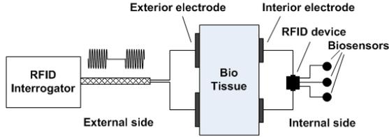
Fig. 2. The proposed volume conduction RFID system.
