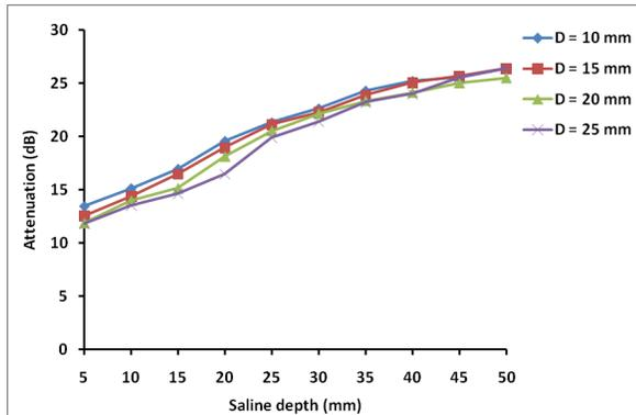
Fig. 7. Signal attenuation with metal sheet using different sizes ( $D$ ) of interior electrodes with 30 mm distance between each center.
