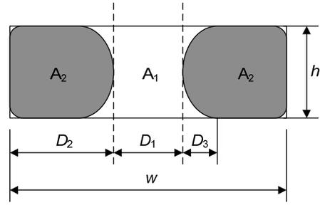
Fig. 8. Shape of electrodes with dimension control parameters.
