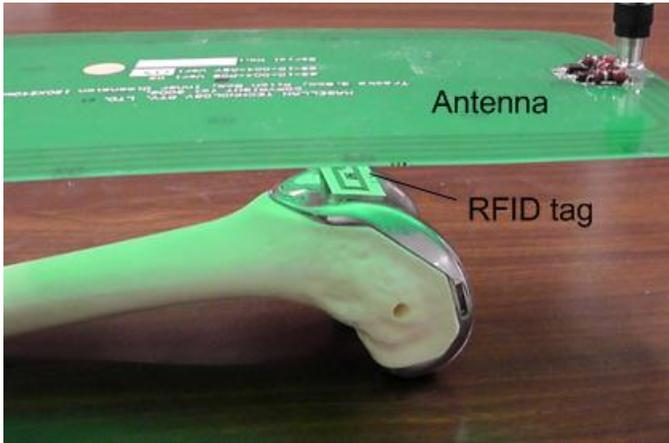
Figure 2. Reading an embedded tag placed on a knee implant using inductive coupling.
