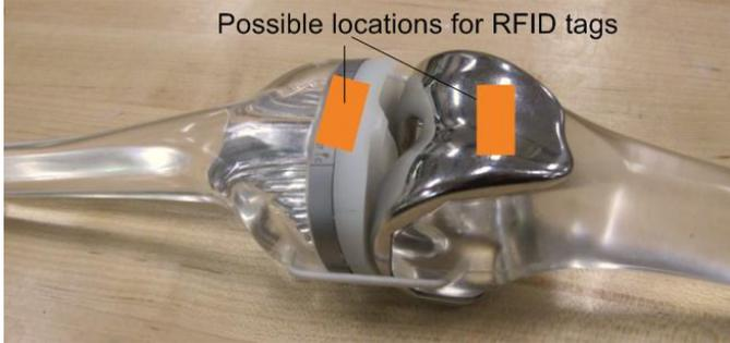
Figure 1. A knee implant with possible locations for RFID tags.
