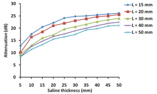
Figure 6. Signal attenuation through saline (D=10 mm).
