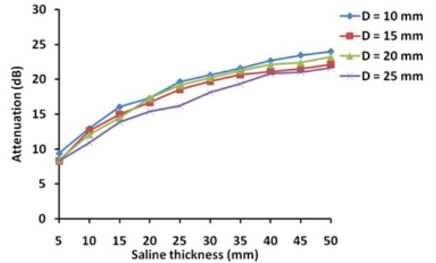
Figure 7. Signal attenuation through saline (L=30 mm).
