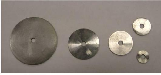
Figure 5. Electrodes in different sizes.
