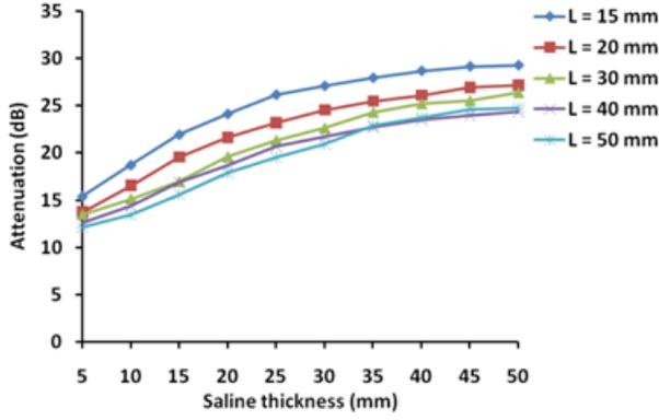
Figure 8. Signal attenuation through saline with metal plate interference (D=10mm).
