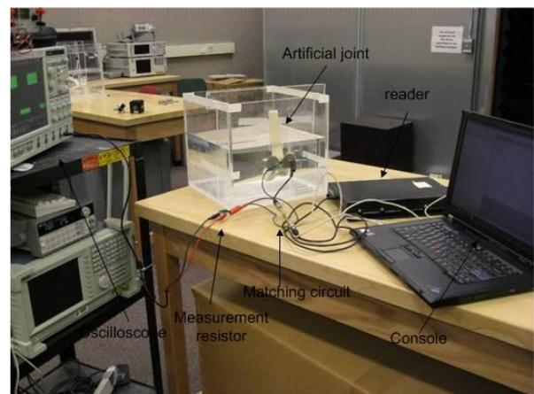
Figure 12. The experiment setup.
