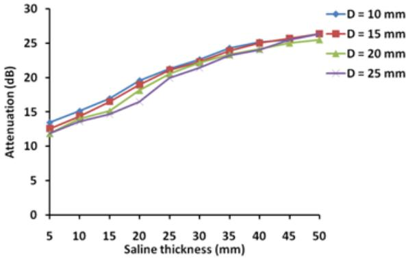
Figure 9. Signal attenuation through saline with metal plate interference (L=30 mm).
