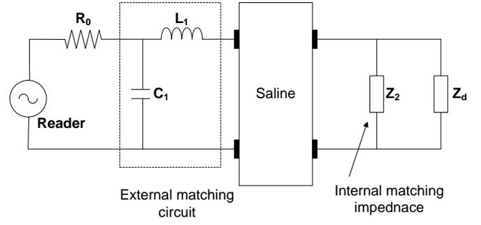
Figure 10. The matching circuit for volume conduction system.
