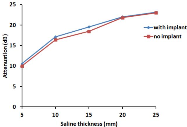
Figure 13. Attenuation with and without a metallic implant using the prototype embedded RFID tag.
