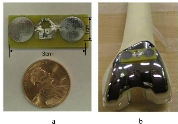
Figure 11. a. The prototype RFID tag and. b. place that the RFID is attached to the implant.
